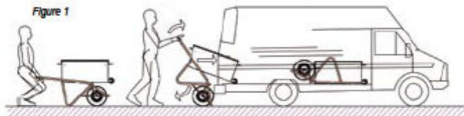
Avoids unnecessary lifting or emptying of the tool wheelbarrow
