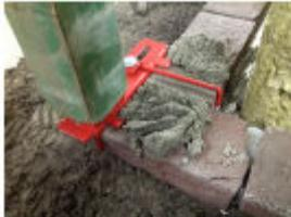
For wall widths of 40 to about 150 mm.
